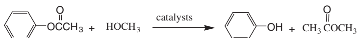
Scheme 1. The transesterification of methanol with phenyl acetate. The products were determined by GC and GC-MS.
